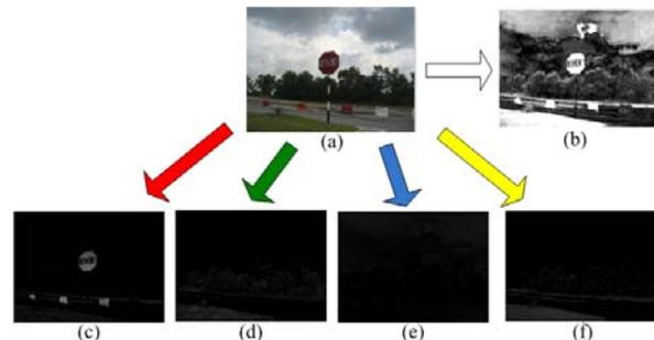
Figure 3. Color segmentation is applied to the (a) input image, to obtain (b) chromaticity, (c) red, (d) green, (e) blue, and (f) yellow color maps.
