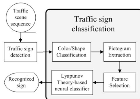
Figure 1. Block diagram of the proposed traffic sign recognition.
