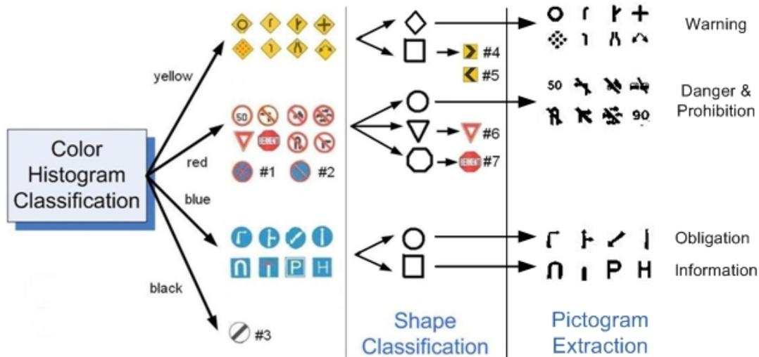
Figure 4. Color histogram, shape classification and pictogram extraction.
