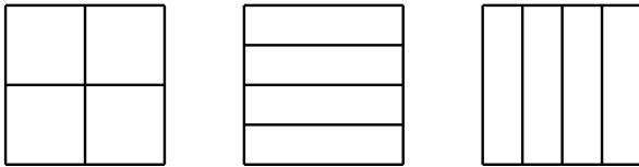
Figure 6: This figure shows the partition of the image block B from the moving window for checking homogeneous regions.
