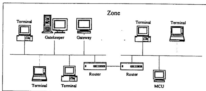
Figure 1: A zone in a mobile IP telephony system
