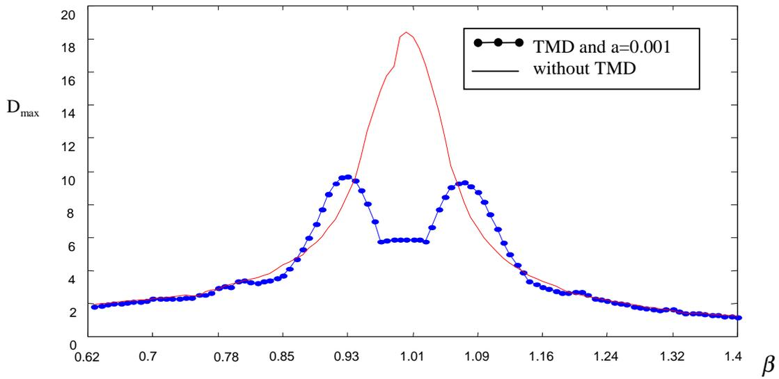
Fig. 4.4. Dynamic magnification factor of a TMD system with nonlinear stiffness  $k(x)$ .
