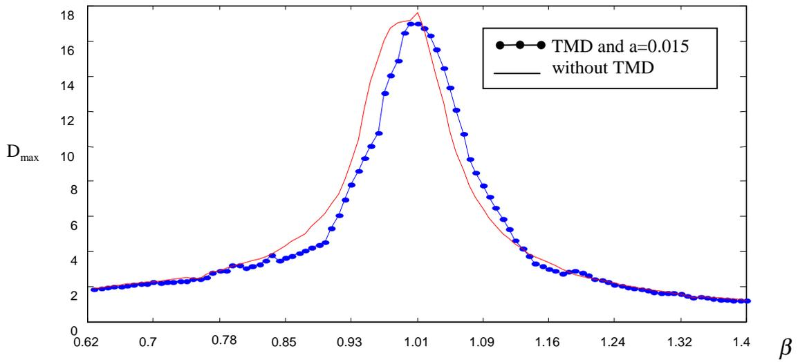
Fig. 4.6. Dynamic magnification factor of a TMD system with nonlinear stiffness  $k(x)$ .
