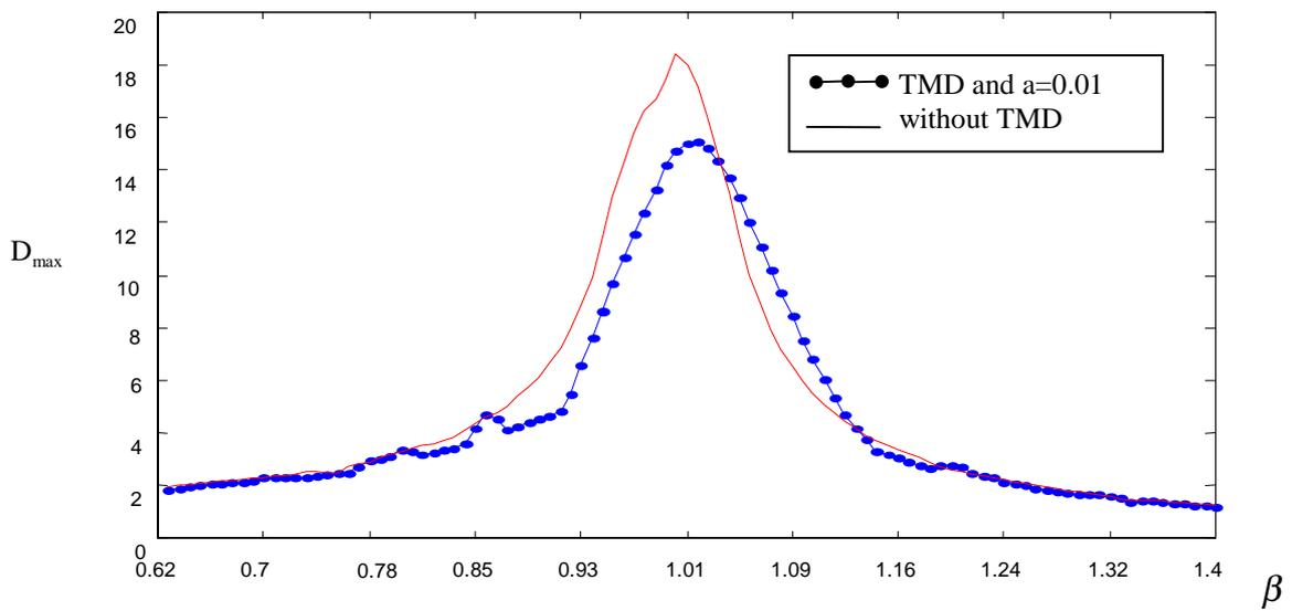
Fig. 4.5. Dynamic magnification factor of a TMD system with nonlinear stiffness  $k(x)$ .
