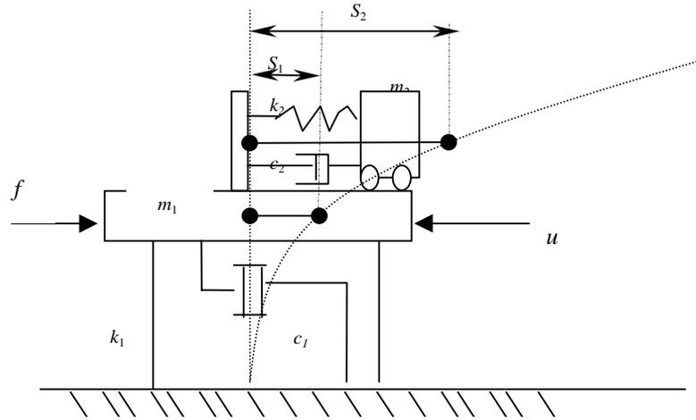
Fig. 4.1. Two-DOF structure-TMD system.
