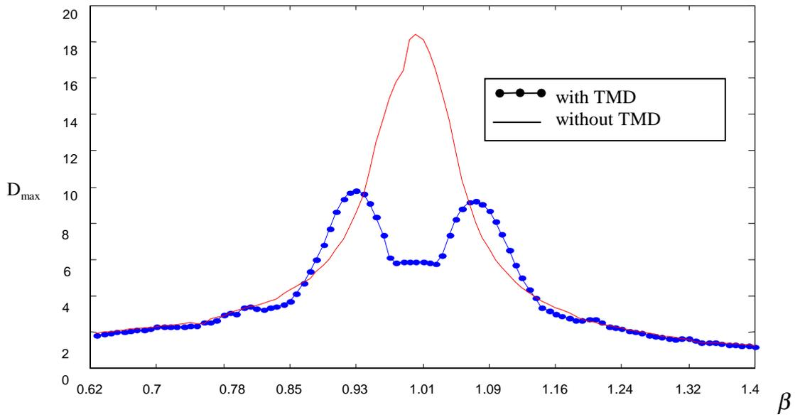
Fig. 4.3. The effectiveness of a TMD system with linear stiffness  $k(x)$ .
