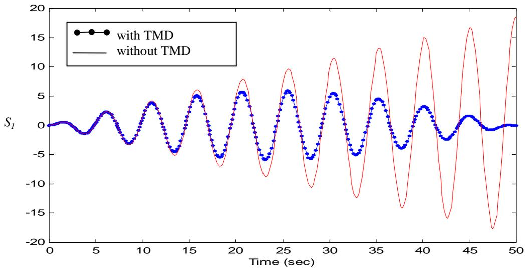
Fig. 4.2. The effectiveness of a TMD system.
