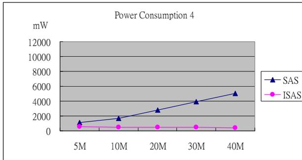
Figure 4-4 : Compare power consumption of SAS and ISAS, wind velocity 0.5 meter per second and diffusion stimulus timing = 300 Second (1)
