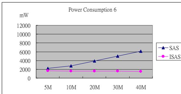
Figure 4-6 : Compare power consumption of SAS and ISAS, wind velocity 0.5 meter per second and diffusion stimulus timing = 900 Second (3)
