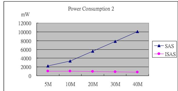
Figure 4-2 : Compare power consumption of SAS and ISAS, wind velocity 0.25 meter per second and diffusion stimulus timing = 600 Second (2)
