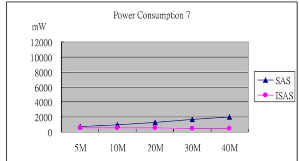
Figure 4-7 : Compare power consumption of SAS and ISAS, wind velocity 1.5 meter per second and diffusion stimulus timing = 300 Second (1)
