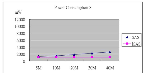
Figure 4-8 : Compare power consumption of SAS and ISAS, wind velocity 1.5 meter per second and diffusion stimulus timing = 600 Second (2)
