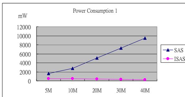
Figure 4-1 : Compare power consumption of SAS and ISAS, wind velocity 0.25 meter per second and diffusion stimulus timing = 300 Second (1)
