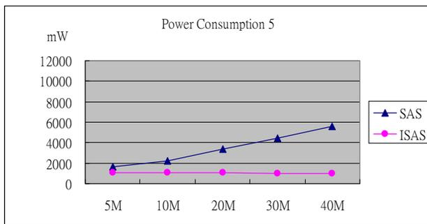
Figure 4-5 : Compare power consumption of SAS and ISAS, wind velocity 0.5 meter per second and diffusion stimulus timing = 600 Second (2)
