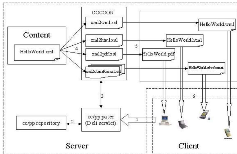
Figure 2. Content adaptation mechanism
